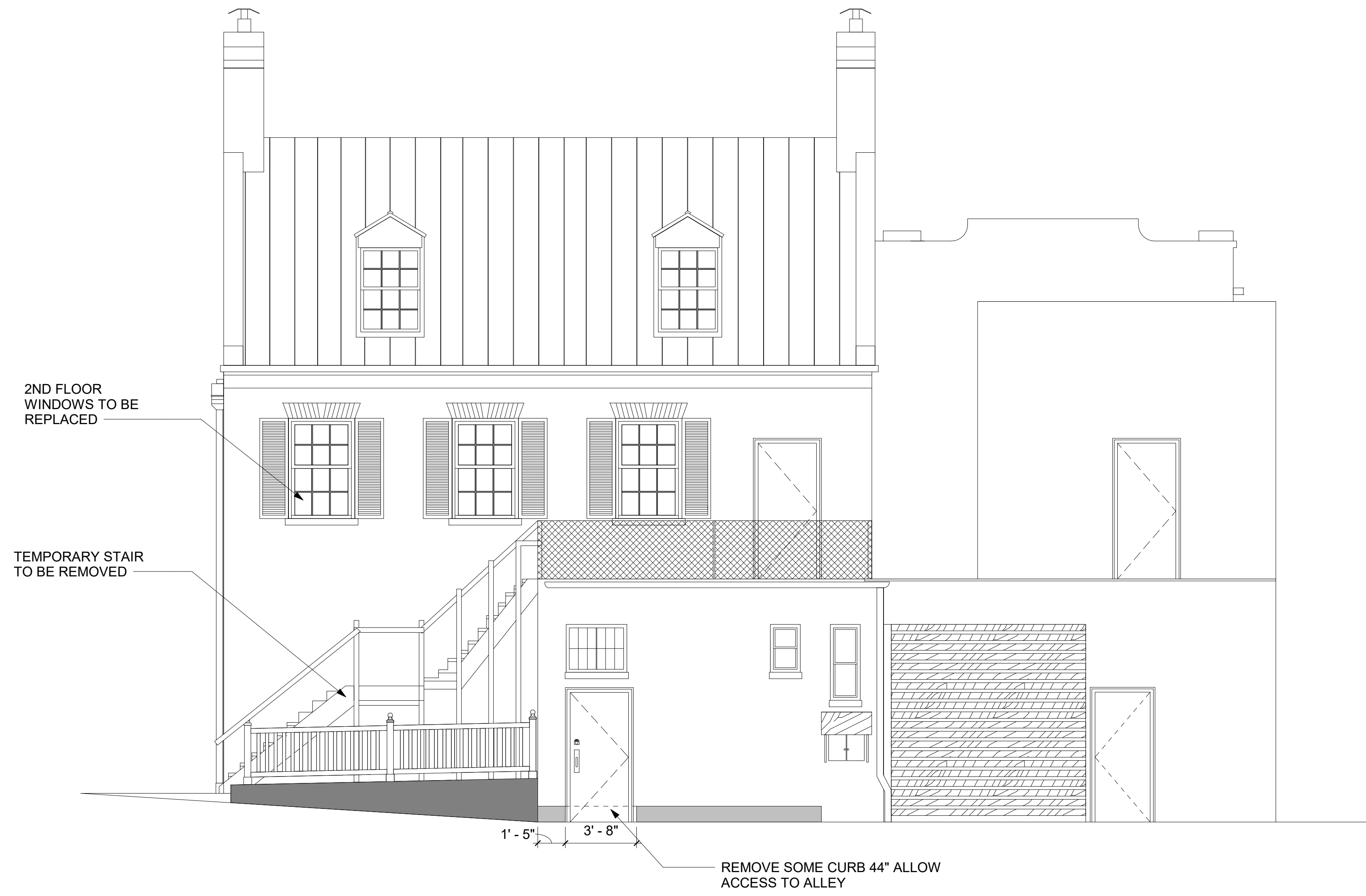
1 EXISTING EXTERIOR REAR ELEVATION - 5' PUBLIC ALLEY A010 / 1/4" = 1'-0"
